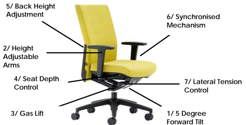
**Seat height adjustment** Establish the right seating height with both the hips and knees comfortable at right angles. To increase the seat height, lift your weight from the seat and pull the lever under the right side of the seat up. To make the chair decrease in height use your body weight, by sitting in the chair at the same time as pulling the lever up. Always release the lever to lock the chair into a comfortable height
